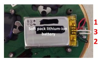
Carefully remove the battery which is held in place by double-sided tape.
