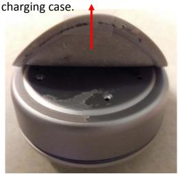
Locate and remove the four screws.
