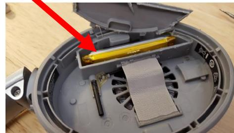
**(B)** Carefully remove the battery which is held in place by double-sided tape.
