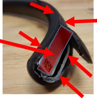
Note the soft pack lithium-ion battery location. Avoid damaging the battery while opening the product.
