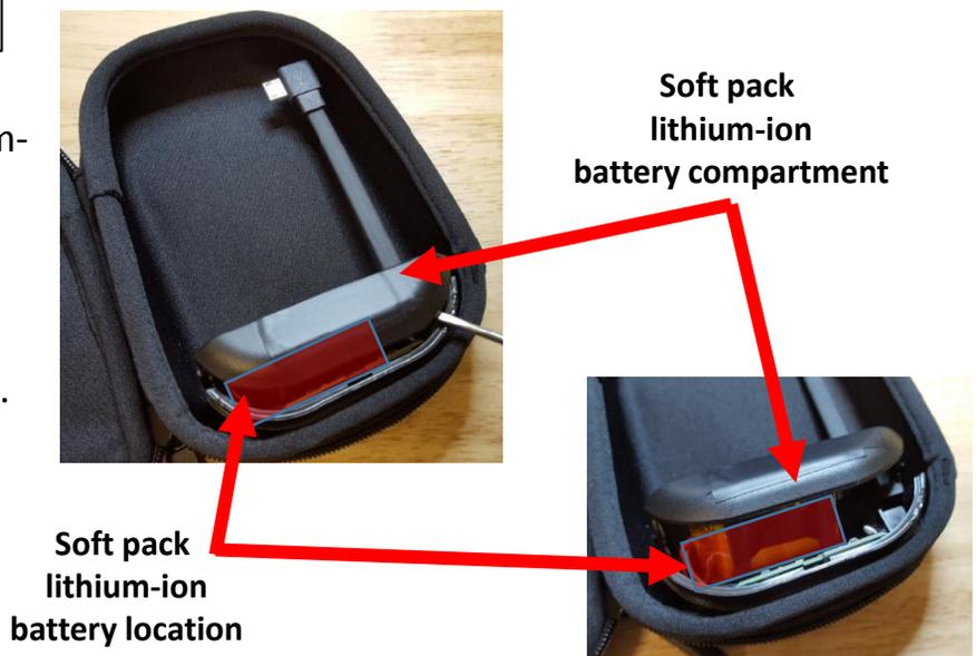
**(B)** Carefully remove the battery which is held in place by double-sided tape.
