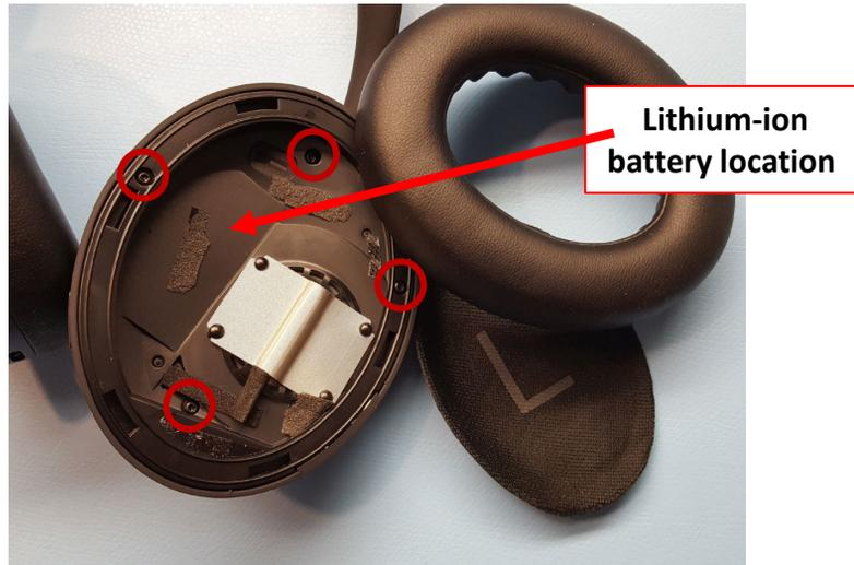
**(C)** Carefully remove the battery which is held in place by double-sided tape.
