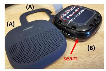
**(C)** Carefully remove the battery from the cavity holding it.
