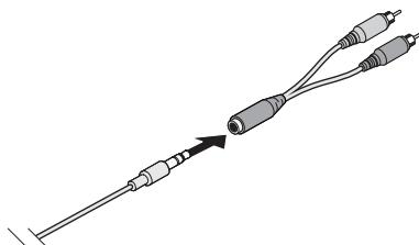
2. Insert the other end of the 3.5 mm audio cable into the **AUX OUT** connector on the Bose® Bluetooth® audio adapter.
