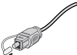
2. Align the plug with the **OPTICAL** connector on the adapter and insert the plug carefully.
