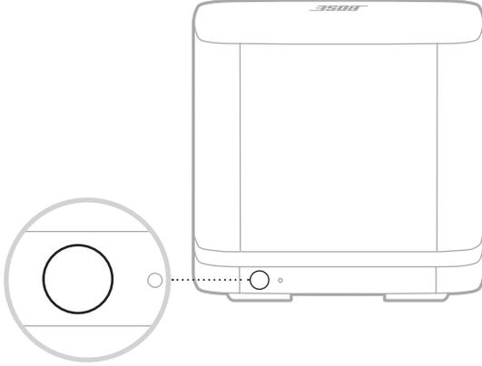
When the bass module reconnects to the soundbar, you hear a tone and the light on the back of the bass module glows white.
