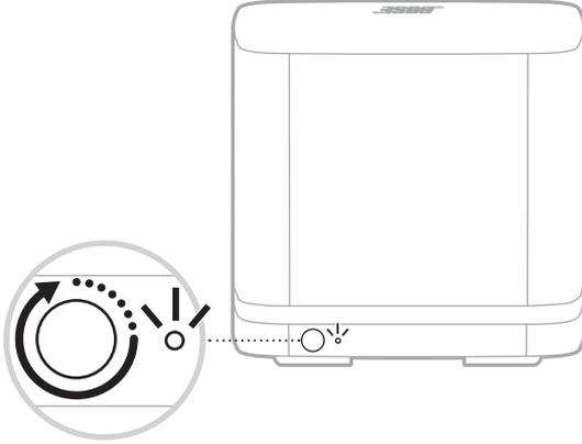
When the reset is complete, the light blinks amber.
