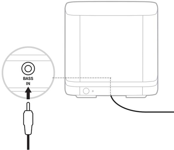
2. Connect the other end of the cable to the **BASS** connector on the back of the soundbar or speaker.
