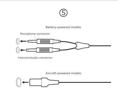
Connect the aircraft connector(s) to the aircraft control panel.
