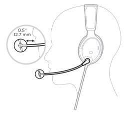
Grasp the microphone base and adjust the boom so the microphone is 0.5" (12.7 mm) from your lips and the white dot on the microphone base is facing your mouth. Insert the AA batteries (2) into the control module.
