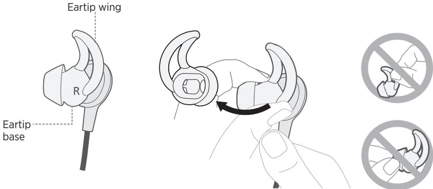
2. Slide the earbud nozzle into the opening of the new eartip, then snap it into place.
