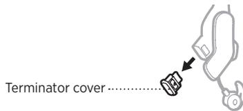
5. On the left side, align the release button to the release button opening, and insert the terminator cover into the base of the connector socket.
