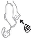
6. Slide the terminator cover into the connector socket until the release button is secure.
