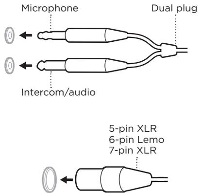
Insert the aircraft connector into the aircraft control panel.
