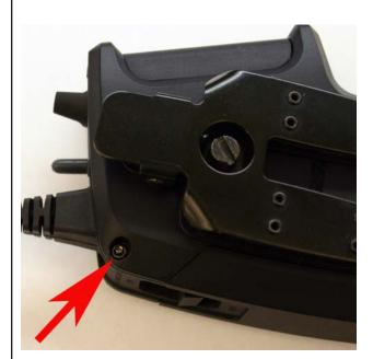
**6.2** On the control module, remove the screw and nut that secure the battery cover. Take care to not lose the small nut. It is not captive to the control module.
