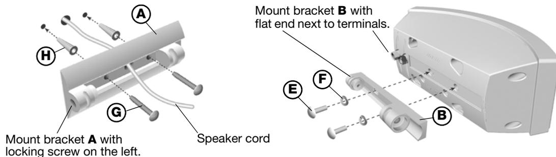
3. Drill holes using the appropriate drill bits for the wall material. Refer to “Required tools and materials” on page 3.
