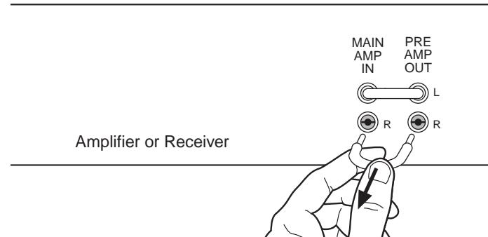
2. Use the twin cable assemblies (with two connectors at each end) that are supplied with the equalizer. Use one connector for the right (R) channel connections and the other connector for the left (L) channel connections.
