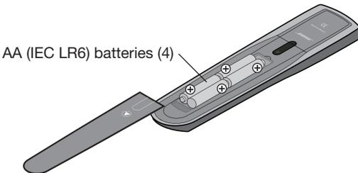
**B.** Install four AA (IEC LR6) batteries, matching the polarity markings (+ and -) to the markings inside the battery compartment.
