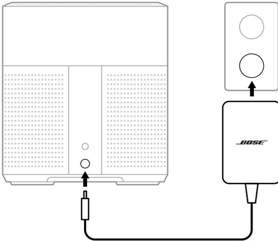
2. Plug the power adapter into an AC (mains) power outlet.
