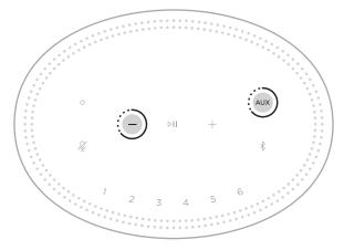
The speaker reboots. When the reset is complete, you hear a tone and the light bar glows solid amber.
