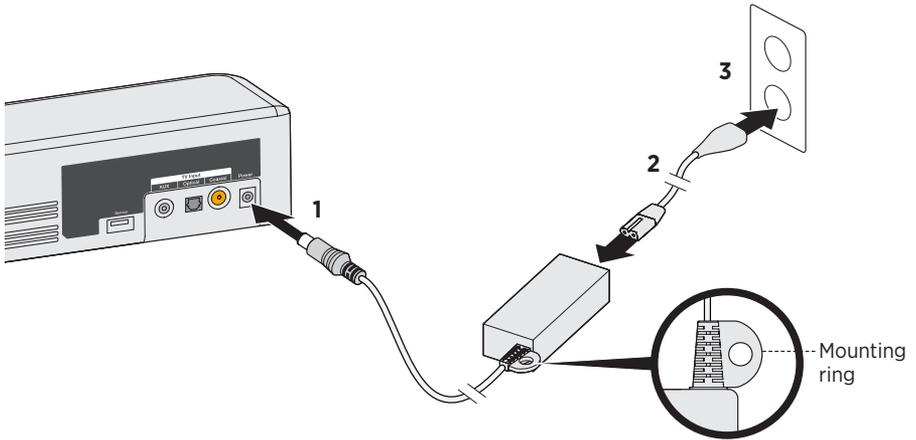
2. Plug one end of the power cord into the power supply.
