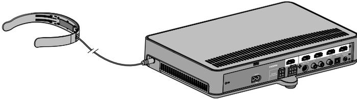
2. Insert the ADAPTiQ headset cable into the
