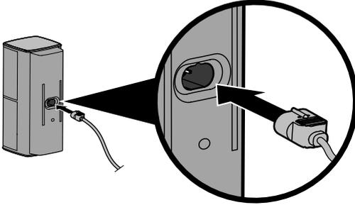
2. Insert the rear speaker cable's **RR** plug into the right rear speaker.
