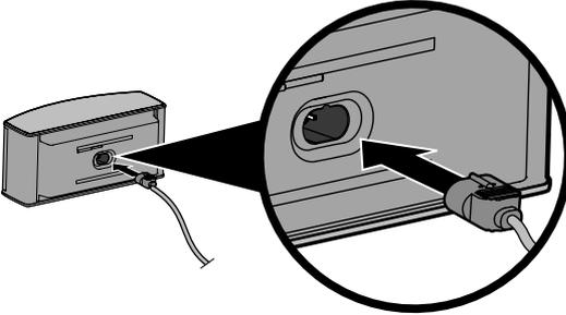
3. Insert the front speaker cable's **R** plug into the speaker on the right of your TV.
