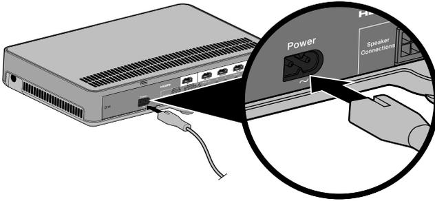
2. Plug the power cord into an AC (mains) outlet.
