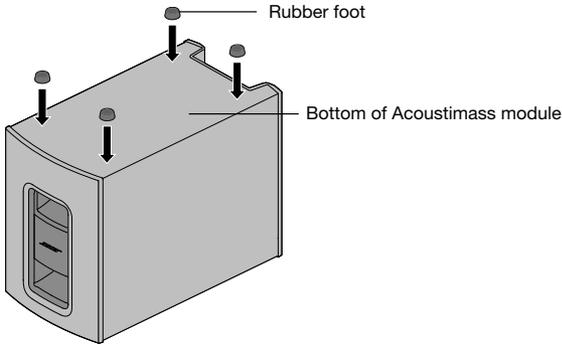
3. Place the Acoustimass module on its feet.
