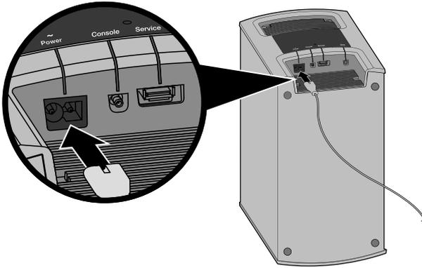
2. Plug the power cord into an AC (mains) outlet.
