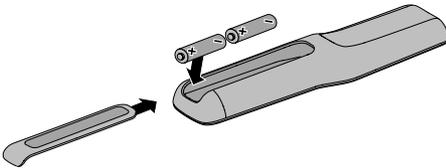
2. Insert the two provided AA (IEC-LR6) 1.5V batteries. Match the + and – symbols on the batteries with the + and – markings inside the compartment.
