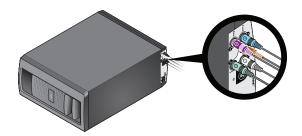
F. Locate the speaker position markings on the free ends of the speaker cables.
