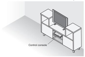
**Note:** Until your system is completely installed, it may be helpful to keep the control console positioned for easy access to its rear connection panel.
