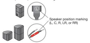
**G.** Using the speaker position markings, run each cable out to its respective speaker as in the following setup example of a room.
