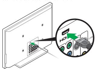
C. Plug the other end of the HDMI cable you are using into the connector labeled **HDMI OUT Video to TV** on the control console.
