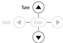
Tunes the FM/AM radio up/down to the next higher/lower frequency.
