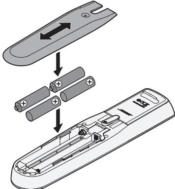
3. Slide the battery compartment cover back into place.
