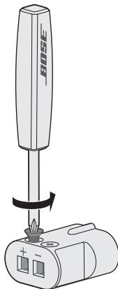
2. **For front speakers:** Insert the bare ends of the four-pin cable into the adapter by placing the red wire marked **L+**, **C+** or **R+** into the red terminal (+) and the plain wire into the plain silver terminal (-).
