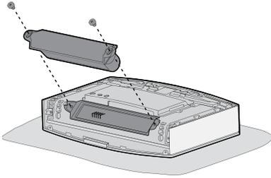
10. Align the cover's hooks to the tabs and press the cover down.
