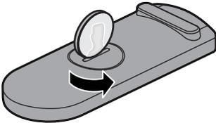
2. Remove the cover. Insert the new battery flat side up, with the + symbol in view.
