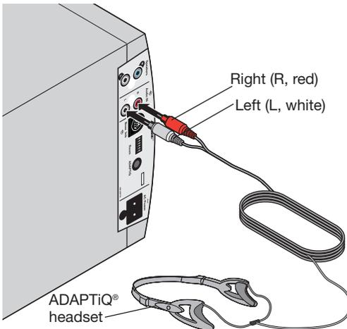
2. Put the headset on your head so the left and right sensors rest above your ears. This headset allows the system to hear exactly what you hear.
