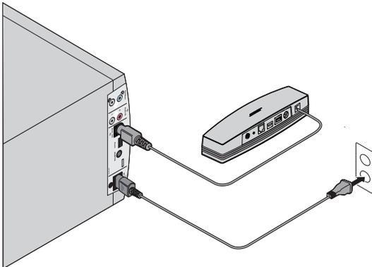
5. Plug the other end of the power cord into AC (mains) power.
