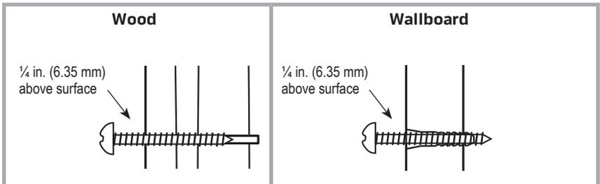
1. Mark holes on the wall 6 1/4 in. (158.7 mm) center-to-center.
