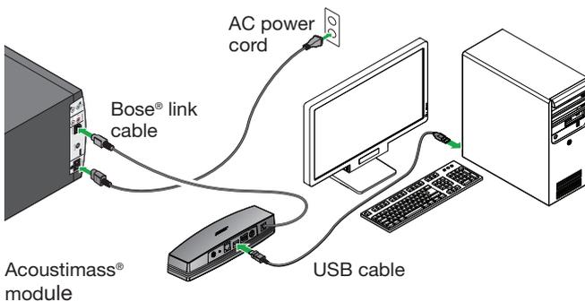
**Note:** Connect the USB cable to the SoundTouch™ wireless adapter only when the app instructs you to do so.
