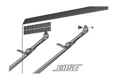
**CAUTION:** The included screws are for use only into wood-studded wall constructions with one-inch (max.) drywall. For all other types of wall construction, please contact a professional installer. Use caution to avoid any electrical or plumbing lines running through the studs.
