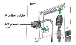
**Note:** You do not need to re-attach the connector cover. Hiding the cables behind the monitor may be easier with the cover removed.
