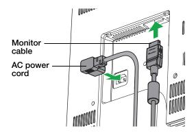
Route both cords through the leg of the stand and re-attach the connector cover.
