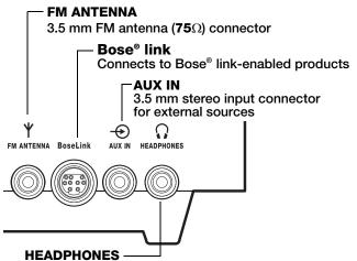
A 3.5 mm stereo headphone connector (system speakers are muted when headphones are connected)
