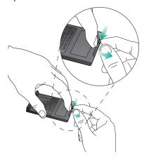
Remove the old battery and install the new one with the plus (+) symbol facing up.
