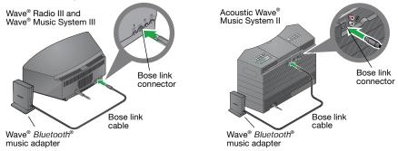
2. Place the adapter in a convenient location. It does not need to be within view. If the adapter is to the left of the system (as you face it), be sure the two are at least 2 in. (5 cm) apart to eliminate any interference with AM reception.
