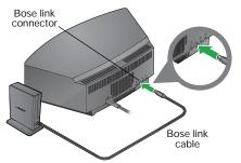
2. Place the adapter in a convenient location. It does not need to be within view. If the adapter is to the left of the system (as you face it), be sure the two are at least 2 in. (5 cm) apart to eliminate any interference with AM reception.
