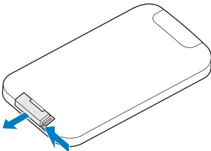
2. Remove the old battery and install the new one with the plus (+) symbol facing up.
