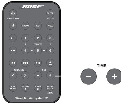
Initially, **HOLD TO SET** appears on the display and then quickly changes to **-CLOCK SET-** as the button is depressed.
