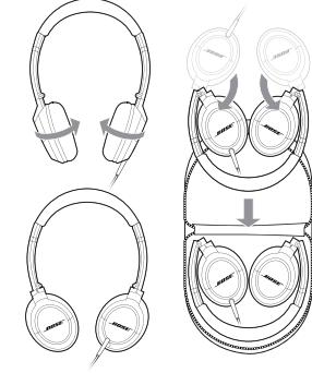
Note: Do not try to exceed the limits of the pivots or over-rotate the earcups.
