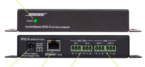
**12VDC input:** +12VDC @ 500mA, center-positive polarity (External supply not required if used with a PoE Ethernet switch)
