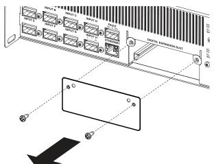
3. Align the Dante card with the plastic card guides in the open slot. Insert the card until the rear panel is flush with the amplifier.
