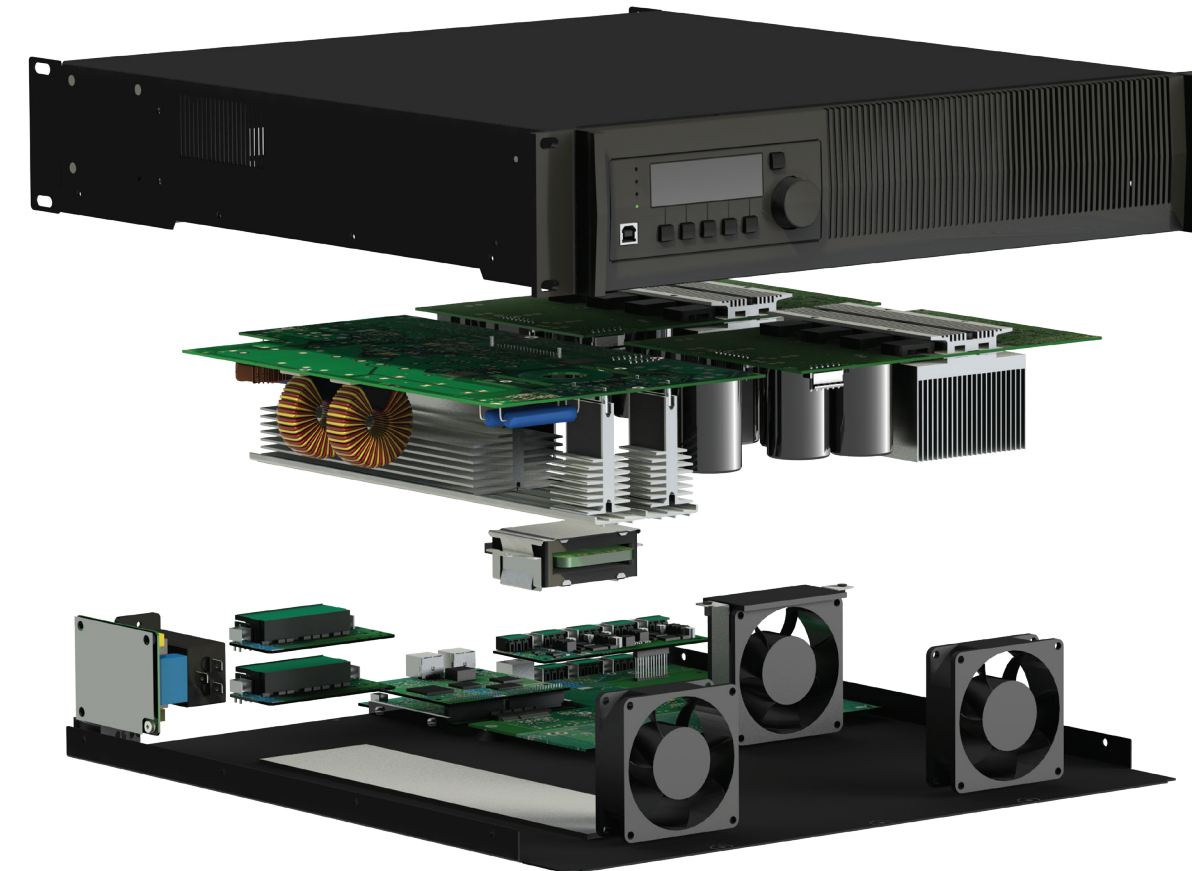
PowerMatch amplifier, internal view
