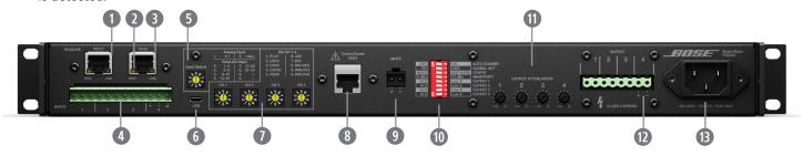
AmpLink - INPUT RJ-45 connector that receives up to 24 digital channels from a Bose AmpLink product. The amp also supports a THRU path for daisy-chaining all 24 digital audio channels to other Bose AmpLink products, at a maximum distance of 10 m between products.
