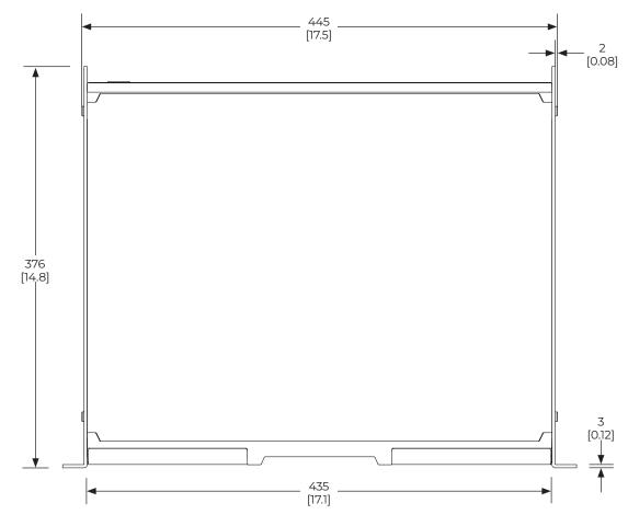
1. DIMENSIONS ARE SHOWN IN MILLIMETERS OVER INCHES. 2. WEIGHT IS APPROXIMATELY 7.0 KILOGRAMS (15.4 POUNDS).
