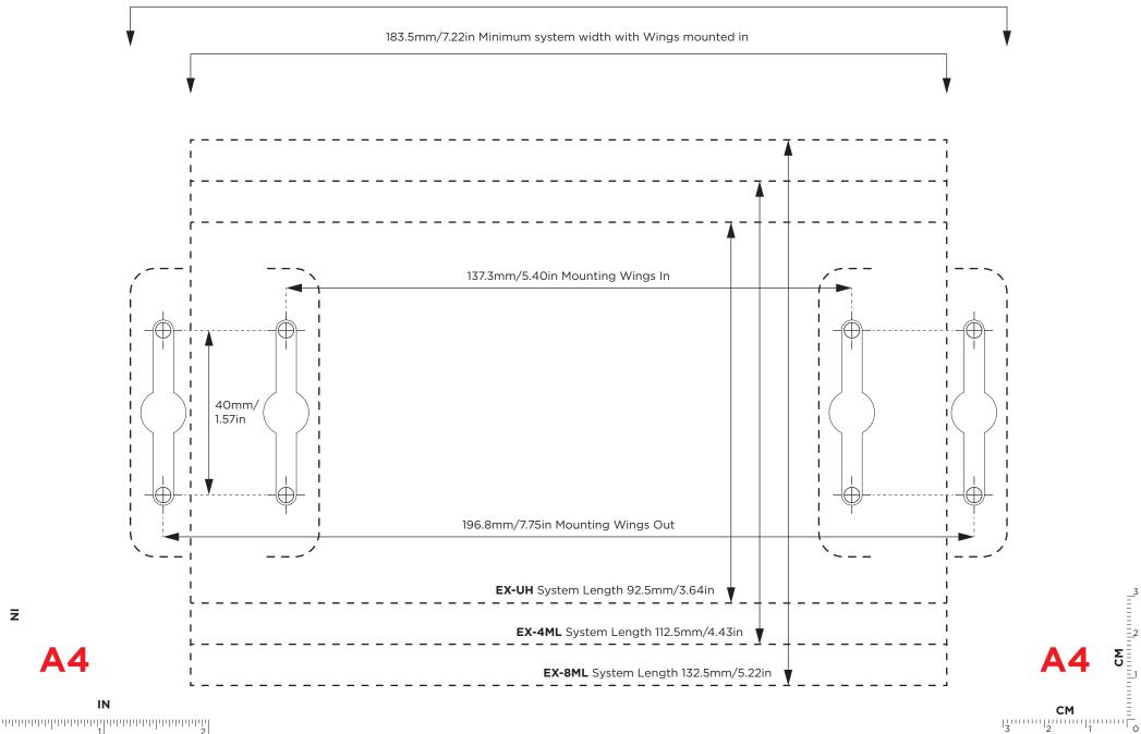
212.8mm/8.38in Maximum system width with Wings mounted out
