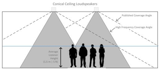
**Figure 2.** To provide a consistent tonal balance across the coverage area in-ceiling loudspeakers must be closely spaced together.
