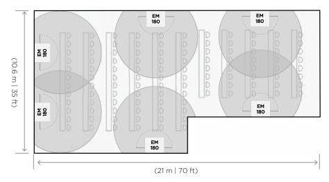
Figure 16. A large conference room with two EM180s mounted near the video screen location, and additional units spaced along room sides using the recommended loudspeaker spacing for the room's ceiling height.
