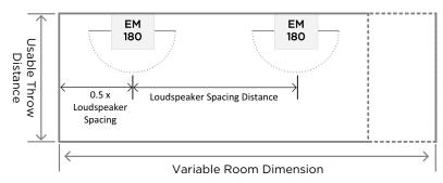
**Perimeter Mounting** - place the EdgeMax loudspeakers along side walls using the spacing distance for the mounting height that will be used.
