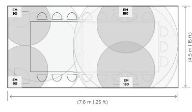
Figure 15. In medium-sized conference rooms two EM90s can be mounted in the front of the room for stereo playback and conferencing, while additional EM180s can be installed along the side walls for conferencing reinforcement.
