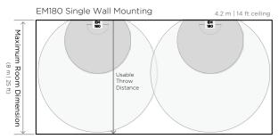
Figure 8. The Maximum Room Dimension is less than or equal to the Usable Throw Distance when EdgeMax loudspeakers are placed along one edge of the area to be covered.
