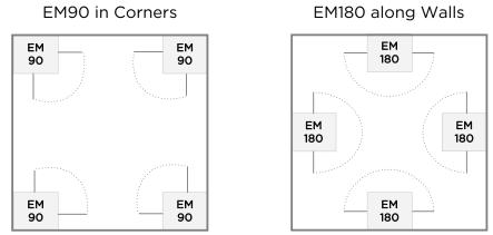
Figure 5. EdgeMax EM90 and EM180 mounting locations.
