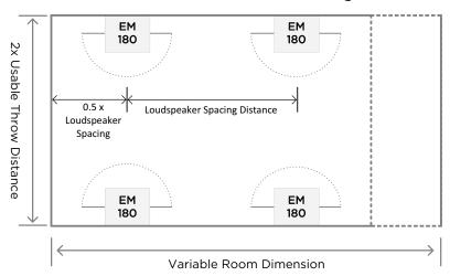
**Mixed (Recommended)** - place the EdgeMax loudspeakers along side walls using the spacing distance for the mounting height that will be used. Follow the guidelines for Single Edge and Perimeter mountings.
