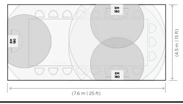
Figure 14. In medium sized conference rooms a single EM180 is used above the screen location, and additional EM180s along the edges provide reinforcement for audio and video conferencing.
