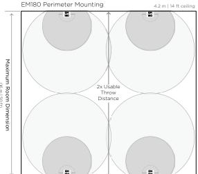
**Figure 9.** The Maximum Room Dimension is equal to twice the Usable Throw Distance when EdgeMax loudspeakers are mounted on two opposing sides of the area to be covered.
