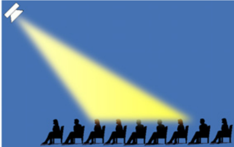
Figure 3b. The effect of choosing a speaker with a radiation pattern narrower than the audience is shown. People outside the main beam get poor sound quality.
