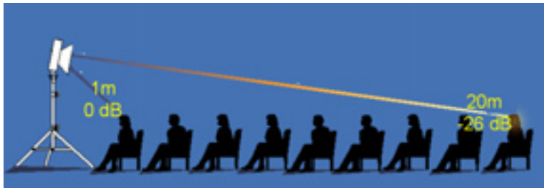
Figure 2a. A traditional speaker producing spherical waves and mounted at ear height in the front of the room results in a 26dB difference in direct field level when the distance ratio of near to far is 1:20. A listener in the back would report the loudness to be four or more times softer than the front.
