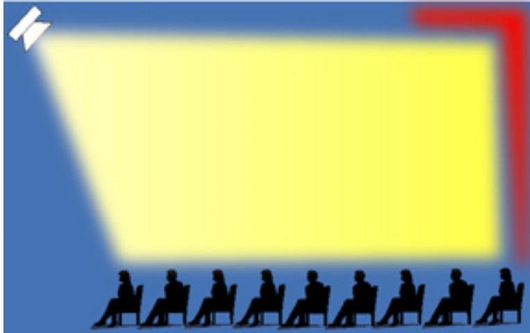
Figure 3a. The effect of choosing a speaker with a radiation pattern wider than the audience is shown. Sound striking surfaces other than the audience causes unwanted reverberation and reduced musical clarity and speech intelligibility.
