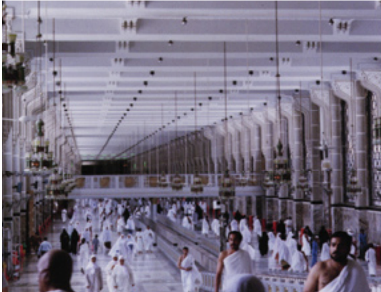
Figure 19. The Massaa area is a long corridor with a reverberation time of about seven seconds. The existing system, along with a wide variety of alternatives explored with Modeler and Auditorer, did nothing to improve intelligibility. A line array solution was tried late in the research phase of the project and proved stunningly effective.
