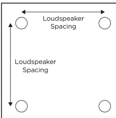
D. After the last loudspeaker is placed, center the loudspeakers in that row to create new offset distances out from each wall, which may be unique from 1/2 LSD.
