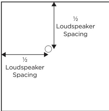
C. The remaining loudspeakers are arranged on a square grid pattern using the LSD. If a loudspeaker would be placed on or beyond the perimeter of the room, delete that row/column of loudspeakers.
