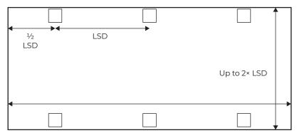
C. After the last loudspeaker is placed, center the loudspeakers in that row to create new offset distances out from each corner, which may be unique from ½ LSD.
