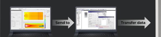
**Bose Professional Array Tool** is the first step in designing the MSA12X into the room. It is a simulation and analysis software that allows audio system designers to define venue parameters, position the MSA12X, and accurately predict its performance.
