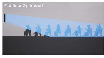
Flat-floor optimized is ideal for flat floor seating with the array bottom slightly above ear height of audience. It provides consistent coverage from the front to the back row.
