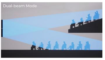
By utilizing all the drivers of the array for both beams simultaneously, dual-beam mode allows you to use any two beam patterns independently.
