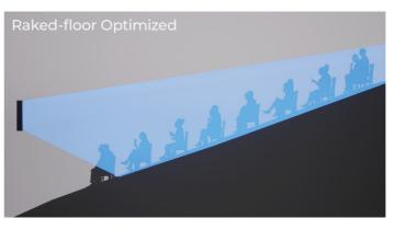
Raked-floor optimized is good for covering a raked floor or flat floor from a relatively high array position. Radiates using a vertically asymmetrical beam.
