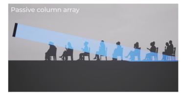
Passive column arrays naturally confine vertical coverage for improved intelligibility and clarity.
