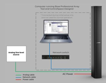
In this configuration, the MSA12X offers a convenient "set it and forget it" approach by receiving an analog line-level source. Once the beam is aimed and programmed, the computer and network switch play a role in the initial setup and can subsequently be disconnected, resulting in a cost-effective analog solution.
