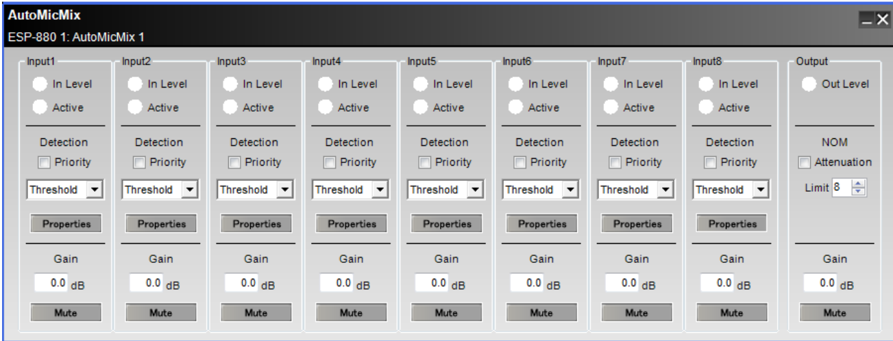
Automatic 8x1 Microphone Mixer processing block and control panel
