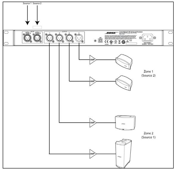
Fig. 5.2- Sample Dual Mono configuration
