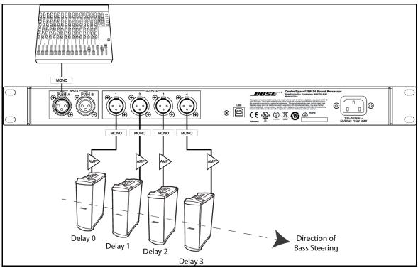
Fig. 5.5- Wiring configuration for an Endfire bass array
