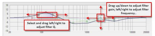
Fig. 3.6- Filter manipulation in parametric mode
