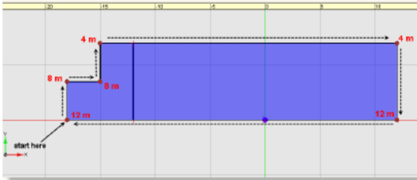
Church ceiling surface with vertex heights
